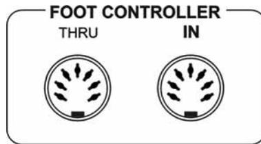
*VENDETTA rear panel Foot Controller MIDI/Channel switching section.*
